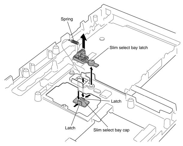
Figure 4-26 Removing the slim select bay latch
